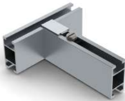
540 - Used where a rail meets on the side of another. The 540 secured with a grub screw and hook securely over the channel of the adjacent profile. Ideal for ceiling grids and bracing rails, page 34
