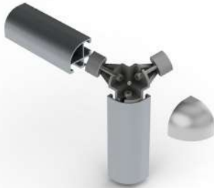
950 - Flex profiles sleeve over 950 universal corner coupling. By adjusting the position of the securing wedge along the arm of the coupling, a friction grip holds the profiles in place. The corner joint is completed by screwing or snap fitting a cap in position, page 38
